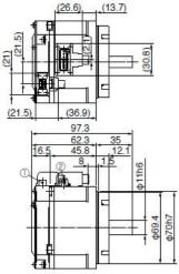
1) Encoder connector ② Motor connector
